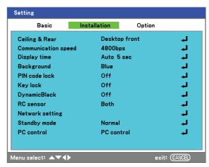
3. Select PIN code lock using ▲or▼. Press ←. You are prompted to enable the PIN code lock function. Select On using ▲or▼. Select OK and press ←.
